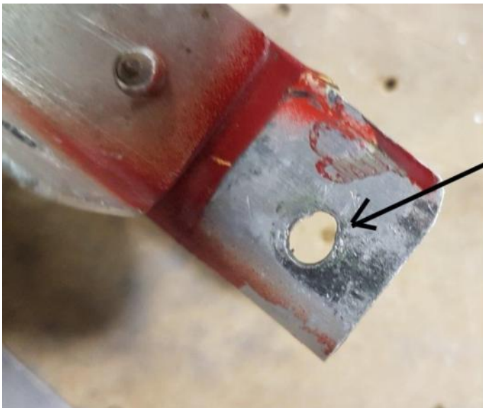
View of H.S. front attachment bracket. Bolt hole was not properly drilled. Part must be replaced.
